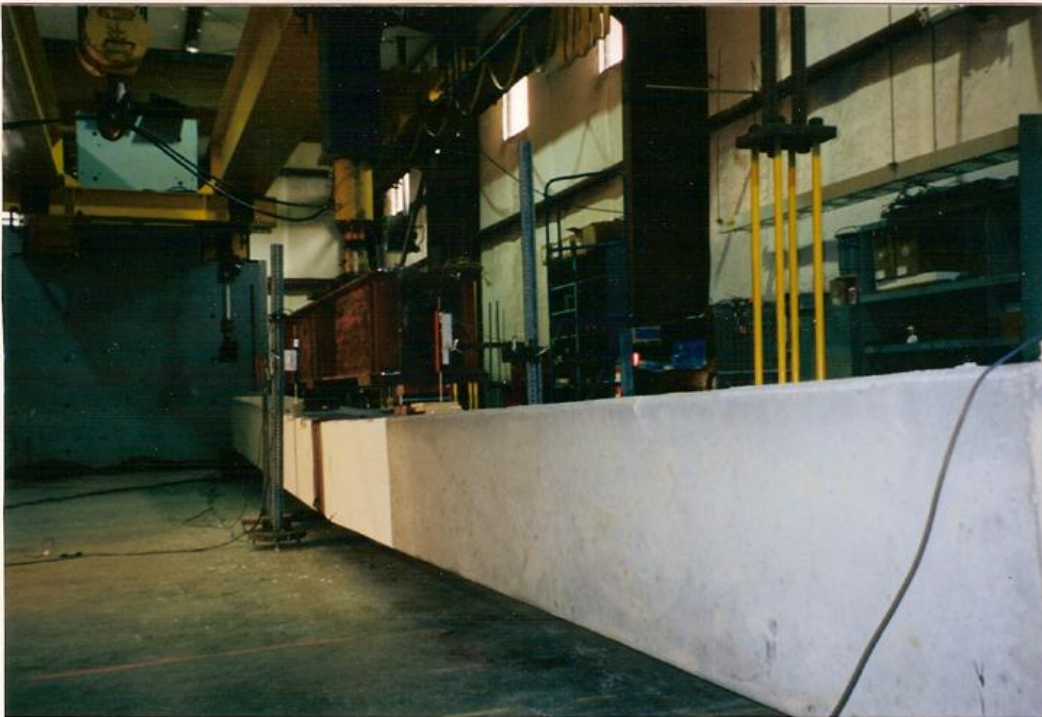
24" Splice Bend Tests, April 2002, FDOT Lab, Tallahassee, verifies ultimate pile capacity of splice
