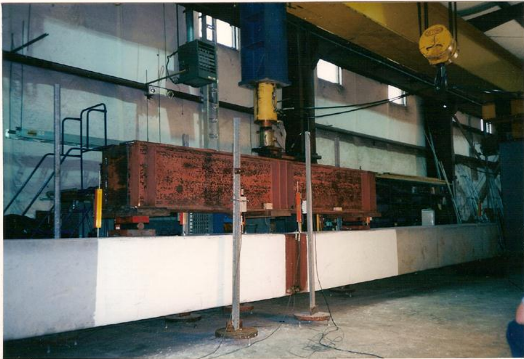
24" Splice Bend Tests, April 2002, FDOT Lab, Tallahassee, verifies ultimate pile capacity of splice
